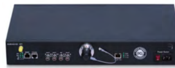
Q4S® Transceiver CCU Fiber Optic Transceiver Video/LAN with optional 12G
