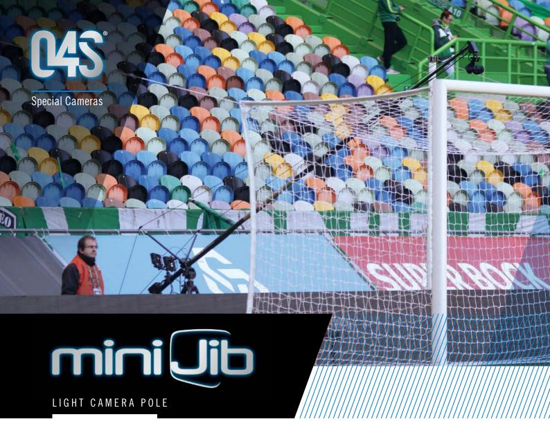
Light camera pole with carbon arm elements that can be assembled in a few minutes to a total length of 5,5m (18.2 ft) and let you move a camera where an ordinary crane cannot be used.
