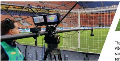
The stabilization corrects all unwanted shaking and vibrations, but also keeps the camera pointed in the same direction, helping operation and delivering rock-steady shots.
